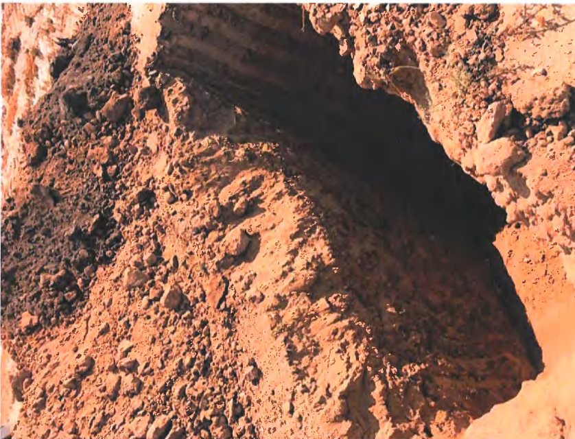
Test Pit #3 - 4'-2" of brown silty sand, then discolored soil mixed with broken asphalt and concrete
