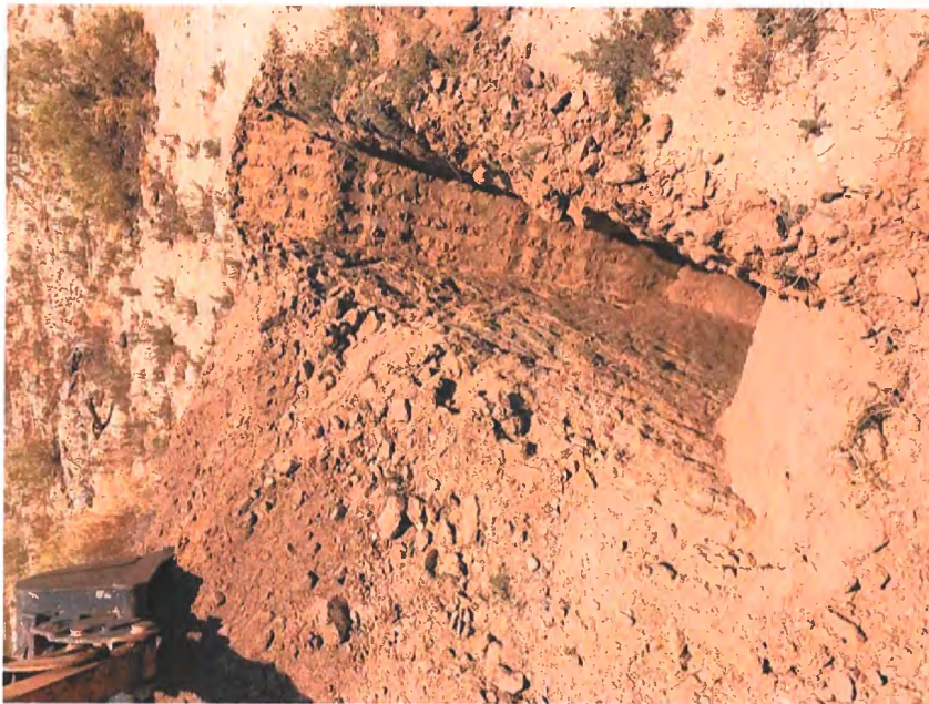
Test Pit #20 - 10'- 0" of brown silty sand (maximum depth of backhoe). This is the soil stockpile adjacent to the bike path. No discolored soil or organics encountered.
