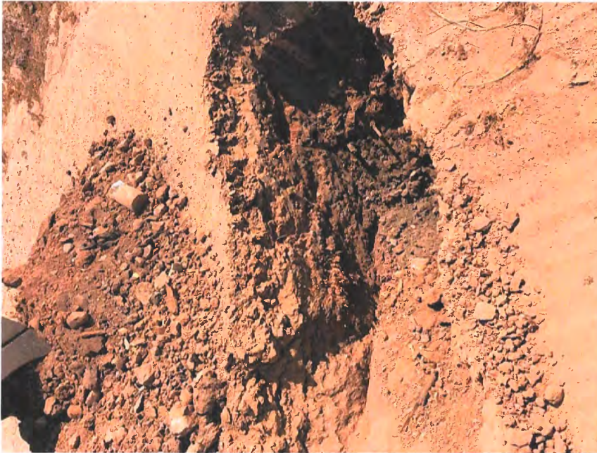
Test Pit #8 – 1'- 0" of brown silty sand, then wood and broken concrete, and concrete test cylinders
