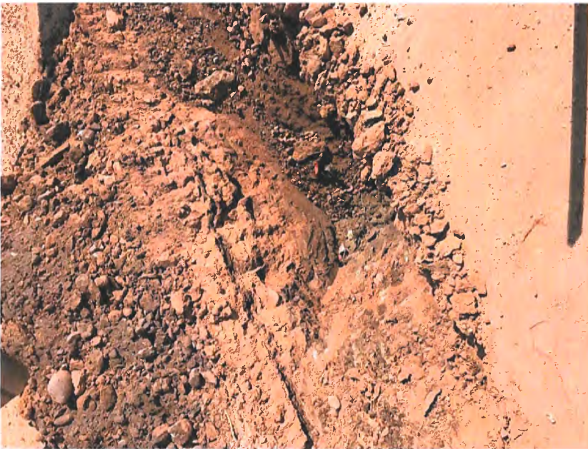
Test Pit #7 – 0'- 10" of brown silty sand, then discolored soil mixed with broken asphalt, plastic and cloth
