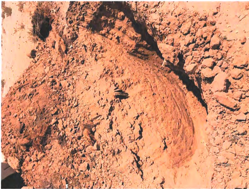
Test Pit #12 – 4'- 6" of brown silty sand, then palm tree waste
