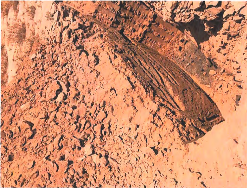
Test Pit #18 – 6'- 3" of brown silty sand, then asphalt millings and discolored soil
