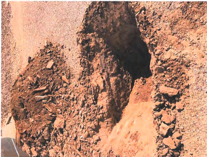
Test Pit #4 - 2' of brown silty sand, then wood and pieces of dimension lumber, with some rock
