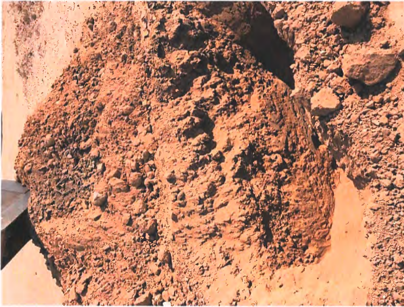
Test Pit #6 – 6'- 1" of brown silty sand, then soil mixed with yard waste trimmings and wood
