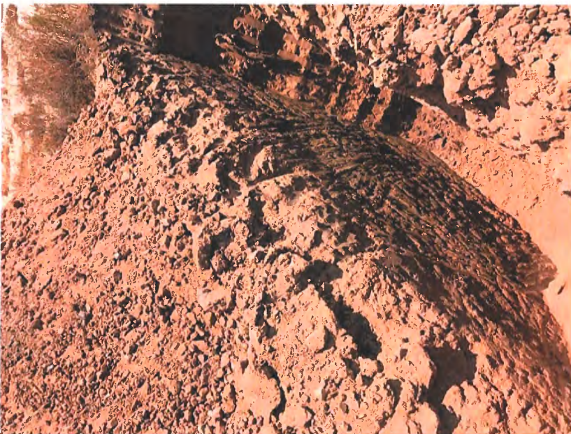
Test Pit #15 – 7'- 10" of brown silty sand, then broken concrete and asphalt and some minor wood waste
