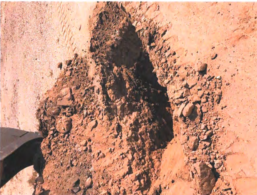
Test Pit #9 – 1'- 6" of brown silty sand, then wood, brick and broken concrete
