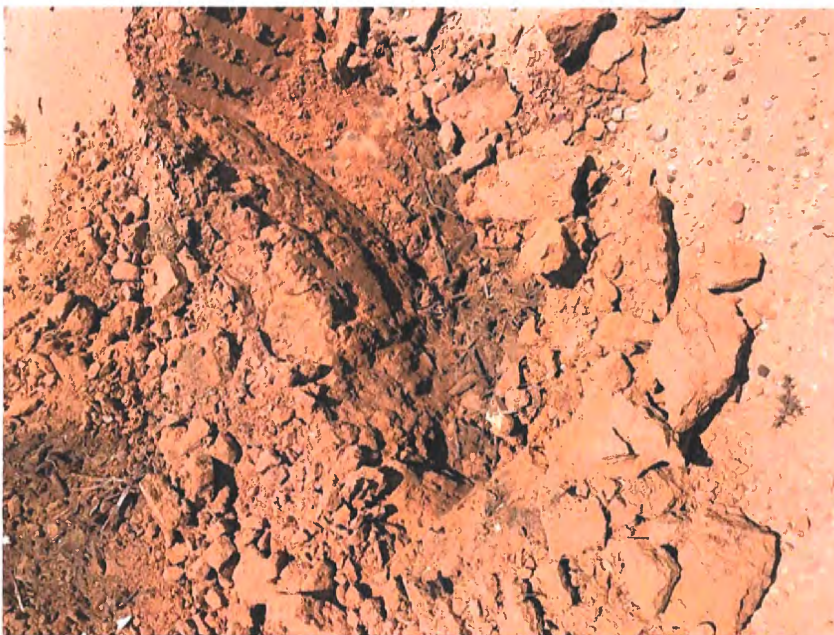
Test Pit #19 – 2'- 6" of brown silty sand, then green waste, stumps and some carpet
