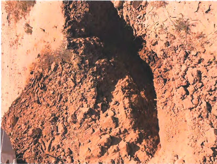
Test Pit #14 – 4'- 0" of brown silty sand, then green waste and tree stumps
