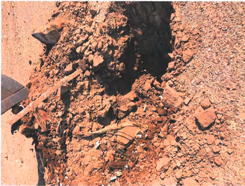
Test Pit #2 - 8' of brown silty sand, then concrete, brick and wood with some metal and wire
