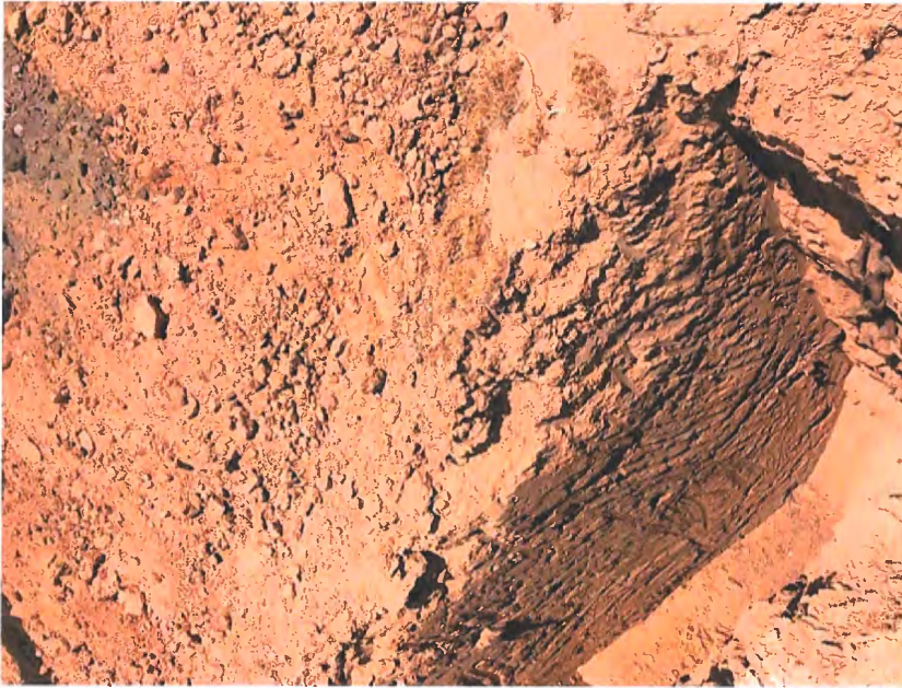
Test Pit #16 – 10'- 0" of brown silty sand (maximum depth of backhoe), then discolored soil with some broken asphalt and plastic waste
