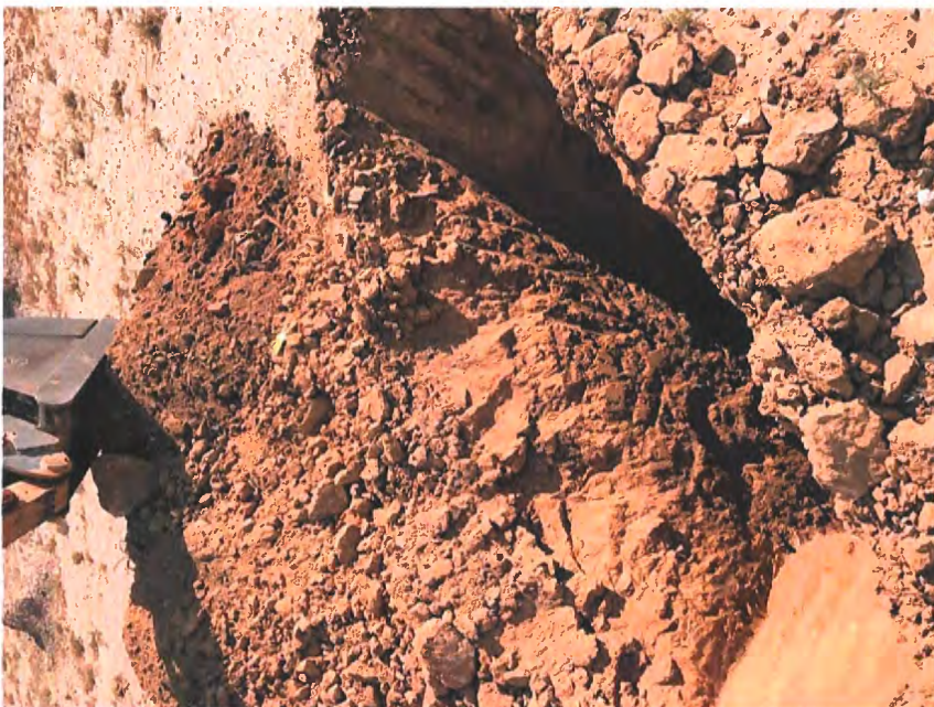
Test Pit #5 - 4'-10" of brown silty sand, then red brick, wire and mixed plastic
