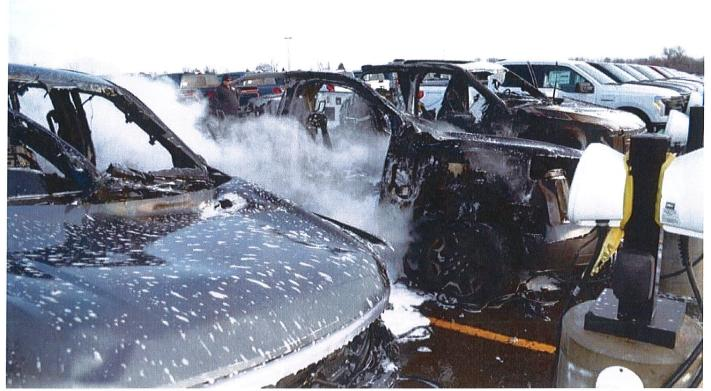
An electric Ford F-150 Lightning caught fire on Feb. 4, 2023 due to a battery issue traced back to one of the automaker's suppliers. The blaze spread to two other electric pickups in a holding lot of Ford's in Dearborn, Michigan.
