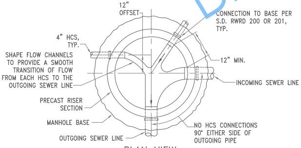
PLAN VIEW (90° MANHOLE IN KNUCKLE INTERSECTION) N.T.S.
