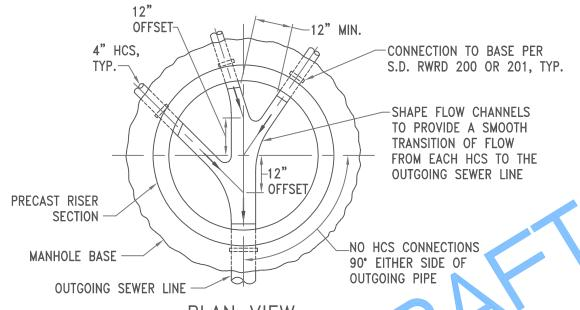
PLAN VIEW (TERMINAL MANHOLE IN CUL-DE-SAC) N.T.S.
