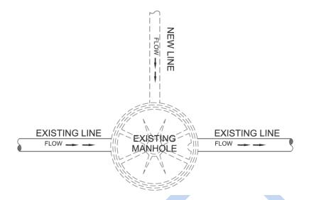
Figure 2-5: New Lateral Sewer Line Connection to Existing Manhole
