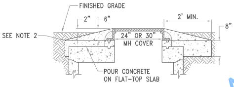
SECTION A-A (FOR FLAT-TOP SLABS)
