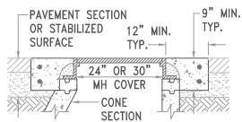
SECTION A-A FOR CONE-TOP N.T.S.
