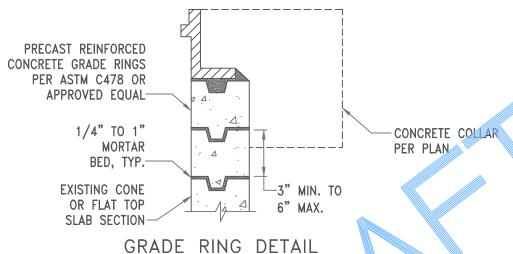
1. A SEWER CONSTRUCTION PERMIT FROM PCRWRD IS REQUIRED PRIOR TO REMOVAL OF THE FRAME AND COVER ON EXISTING PUBLIC MANHOLES. GRADE ADJUSTMENT WORK SHALL BE INSPECTED AND APPROVED BY THE FIELD ENGINEER.
