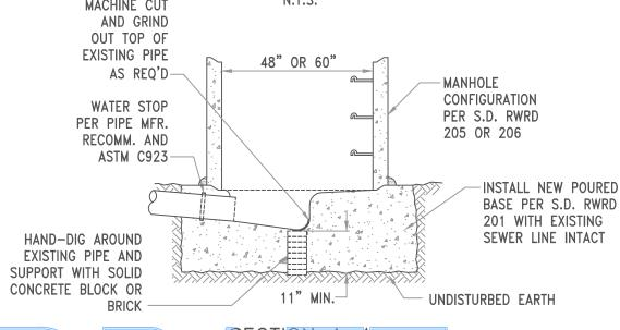
1. FOUNDATION PER S.D. RWRD 104 TO THE FIRST JOINT BEYOND OPEN TRENCH CONDITIONS MAY BE REQUIRED DEPENDING ON DEPTH OF EXCAVATION AND TYPE OF SOIL.
