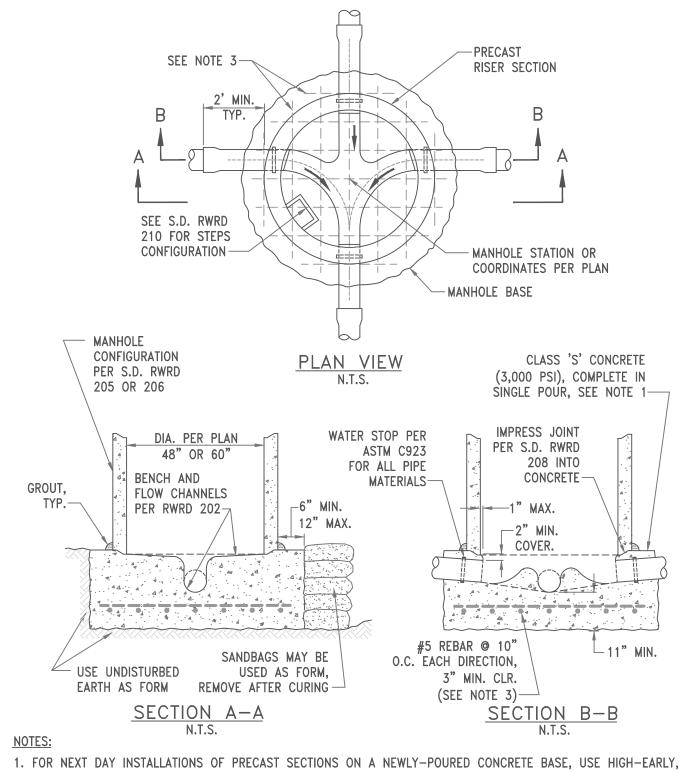
1. FOR NEXT DAY INSTALLATIONS OF PRECAST SECTIONS ON A NEWLY-POURED CONCRETE BASE, USE HIGH-EARLY, CLASS 'S' CONCRETE HAVING A MIN. COMPRESSIVE STRENGTH OF 2,000 PSI AT 24 HOURS AS DEMONSTRATED BY LABORATORY TESTING OF SAMPLE CYLINDERS.
