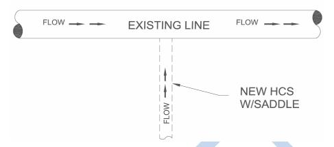
Figure 2-2: Direct Connection to Existing Sewer Lines
