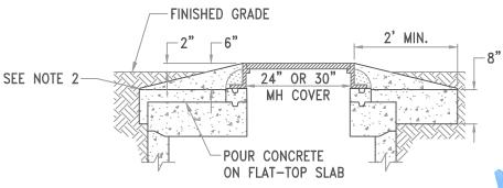
SECTION A-A (FOR FLAT-TOP SLABS)
