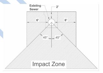
Figure 2-1: Impact Zone for Existing Sewer Lines
