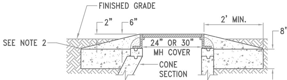
SECTION A-A (FOR CONE SECTIONS)
