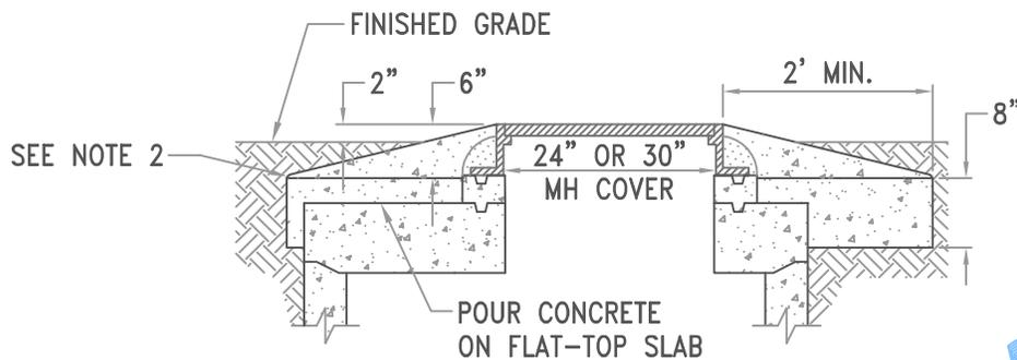
SECTION A-A (FOR FLAT-TOP SLABS)
