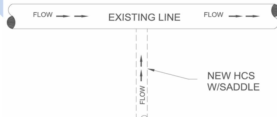
**Figure 2-2: Direct Connection to Existing Sewer Lines**
