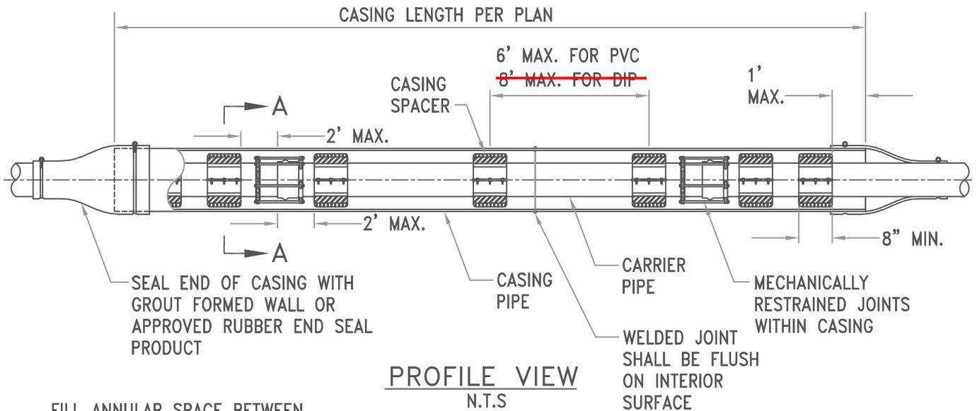
FILL ANNULAR SPACE BETWEEN CASING AND CARRIER PIPE WITH SAND OR  $\frac{3}{8}$ " PEA GRAVEL UNLESS OTHERWISE INDICATED ON THE PLANS OR APPROVED BY THE FIELD ENGINEER
