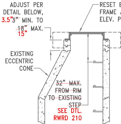
**PRECAST MANHOLE WITH CONE SECTION**
