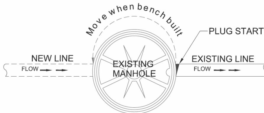
**Figure 2-4: New Sewer Line Connection to Existing Manhole**
