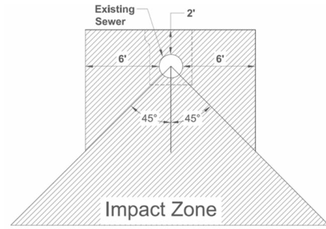
Depending on the sewer type, size, condition, and flow volume, RWRD Field Engineering may increase the Impact Zone. Field Engineering will make the determination at the time of plan submittal.
