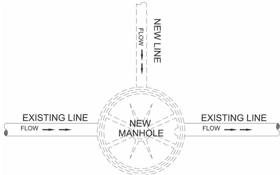
**Figure 2-3: New Manhole on an Existing Sewer Line**
