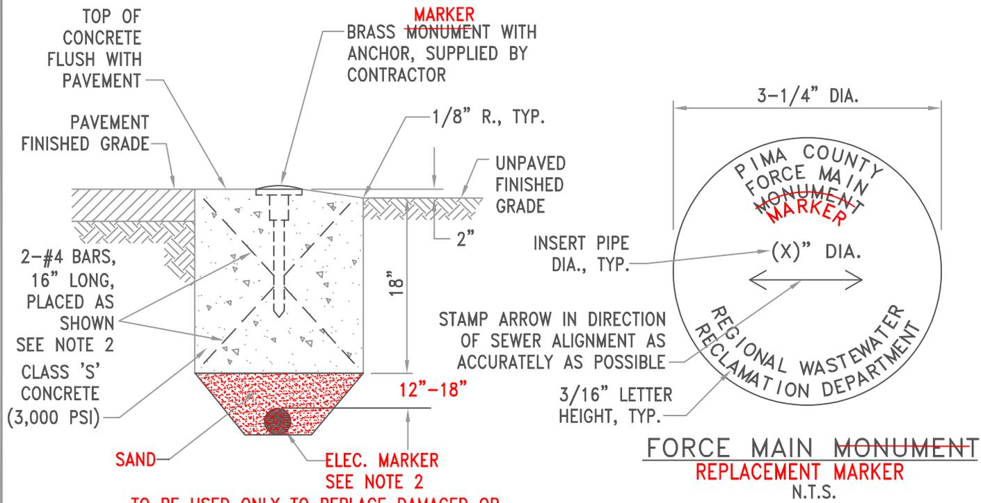
**TO BE USED ONLY TO REPLACE DAMAGED OR REMOVED EXISTING FORCE MAIN MARKERS !**
