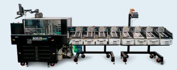
The Agilis can scan ballot envelopes capturing the voter's signature, presenting the image to the user on-screen for signature comparison against the signature from the voter registration database. Challenged ballots such as envelopes with no signature, are identified and separated for manual review. Additionally, if the jurisdiction would require the ability for automated signature recognition, the Agilis provides that option.
