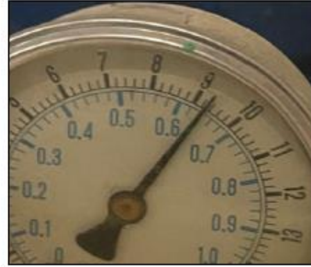
Supporting Data ECM-1 - Blower are operating at about 9.3 psi, base on photo from site visit
