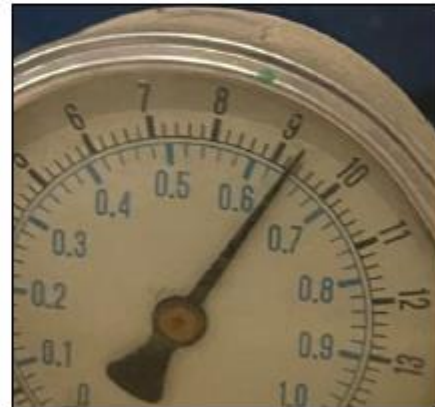
Supporting Data ECM-1 - Blower are operating at about 9.3 psi, base on photo from site visit
