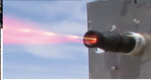
2nd Stage Engine (500 lbf.) Test
