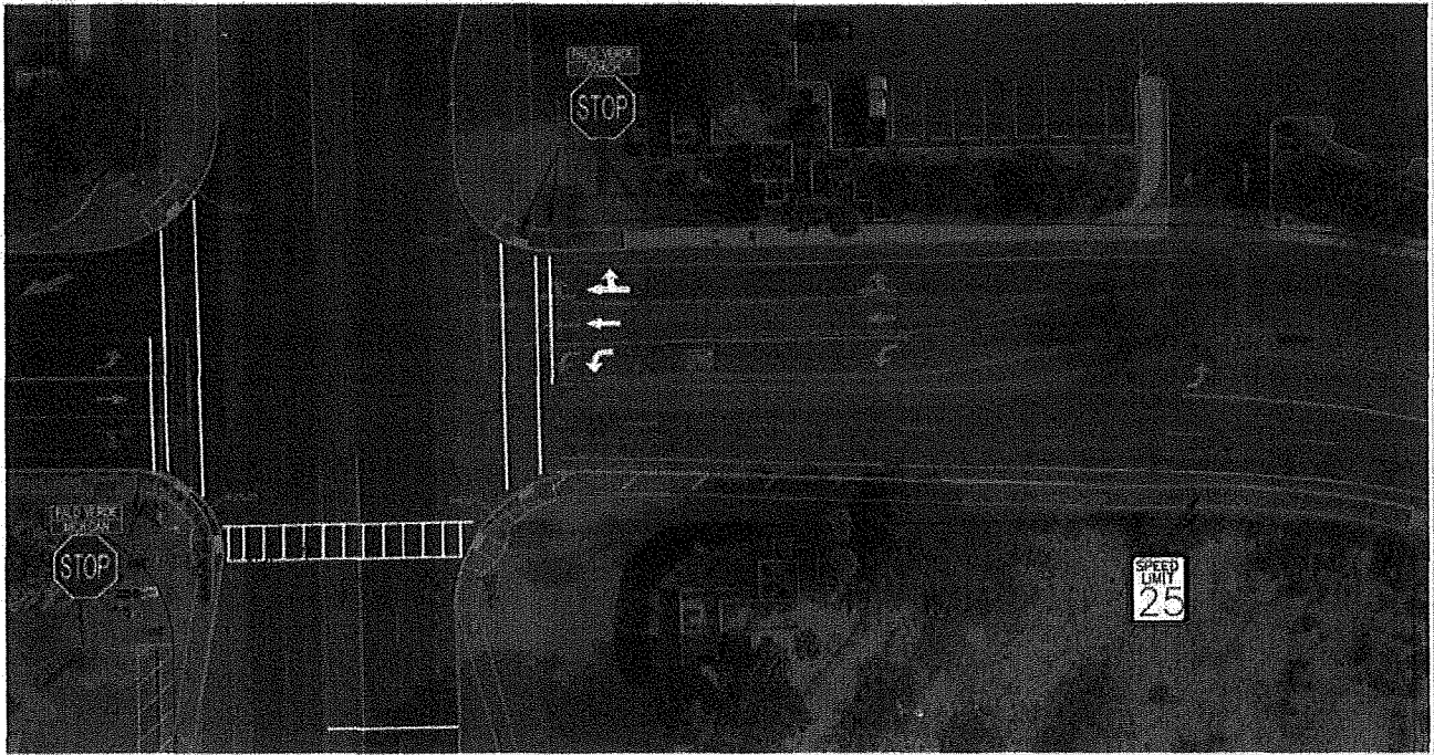
Figure 2 – Conceptual Design of Palo Verde Road and Michigan Street PHB/HAWK
